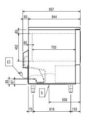
Drain Electrical inlet (power) ΕI Refrigerant Outlet
